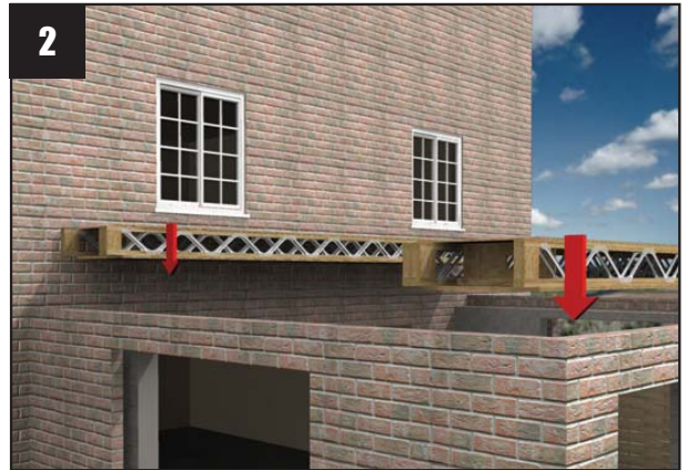
Place the lateral structural cassettes A & B on the inner leaf of the cavity wall. Ensure adequate lifting capacity - eg. Genie Lifts.
