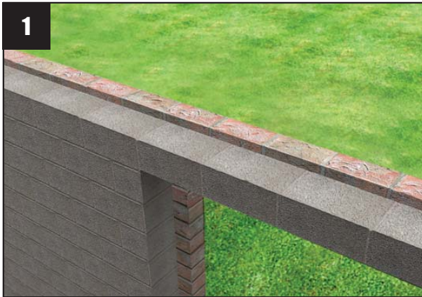
Complete the walls to 1 brick above the lintel on both leaves of masonry. (Lintel missing to ensure clarity of image.)
